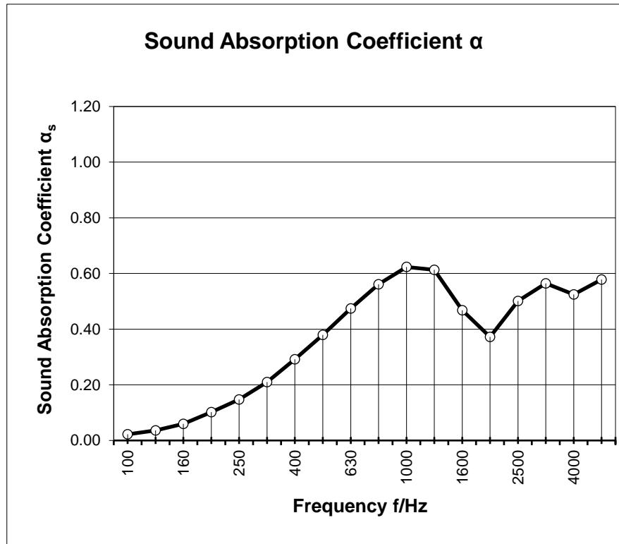
\*Method reproduces conditions, dimensions, build-up in a way results are comparable with measurements in reverberation chamber as Sound absorption coefficient to ISO 354
