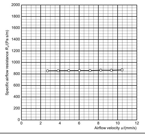
Specific airflow resistance  $R_s(0.5 \text{ mm/s}) = 847 \text{ Pa s/m}$
