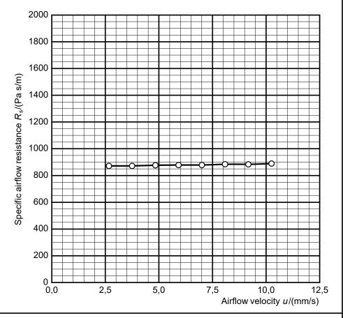
Specific airflow resistance  $R_s(0.5 \text{ mm/s}) = 864 \text{ Pa s/m}$
