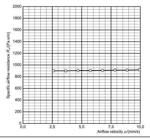
Specific airflow resistance  $R_s(0.5 \text{ mm/s}) = 893 \text{ Pa s/m}$
