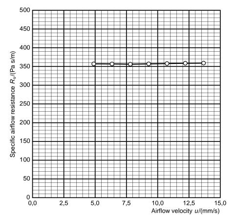
Specific airflow resistance  $R_s(0.5 \text{ mm/s}) = 354 \text{ Pa s/m}$
