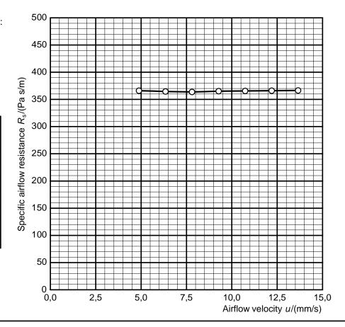
Specific airflow resistance  $R_s(0.5 \text{ mm/s}) = 363 \text{ Pa s/m}$
