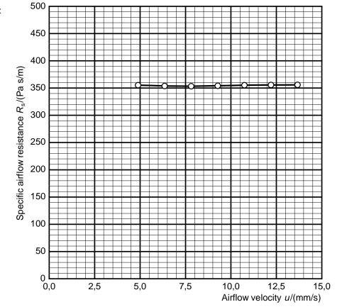
Specific airflow resistance  $R_s(0.5 \text{ mm/s}) = 352 \text{ Pa s/m}$
