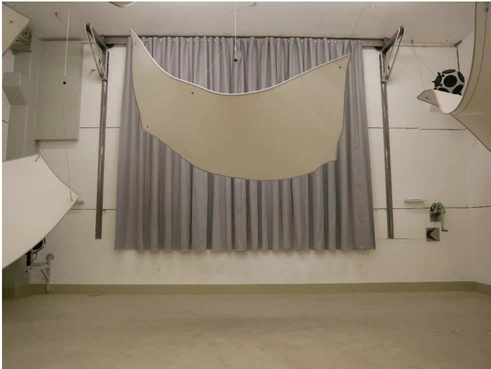
Figure B.3. Pleated hanging curtain, 100 % fullness in the reverberation room: frontal view.
