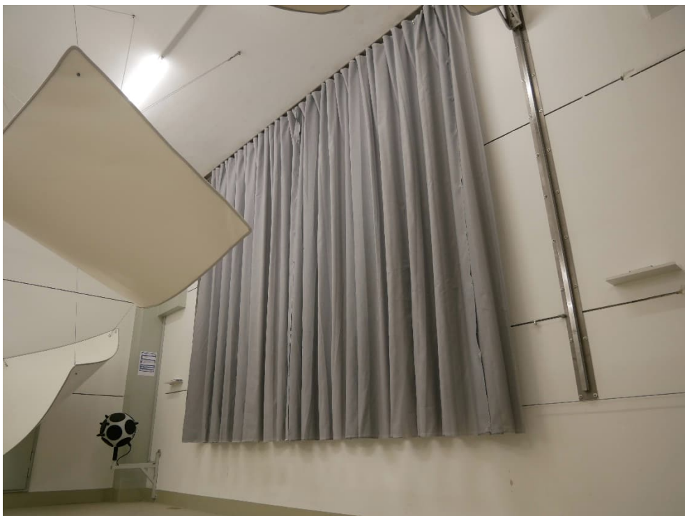
Figure B.4. Pleated hanging curtain, 100 % fullness in the reverberation room: diagonal view.
