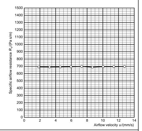
Specific airflow resistance  $R_s = 689 \text{ Pa s/m}$
