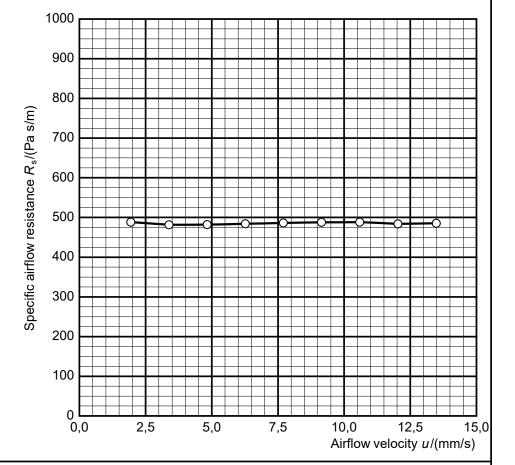
Specific airflow resistance  $R_s$  = 484 Pa s/m
