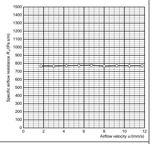
Specific airflow resistance  $R_s = 770 \text{ Pa s/m}$
