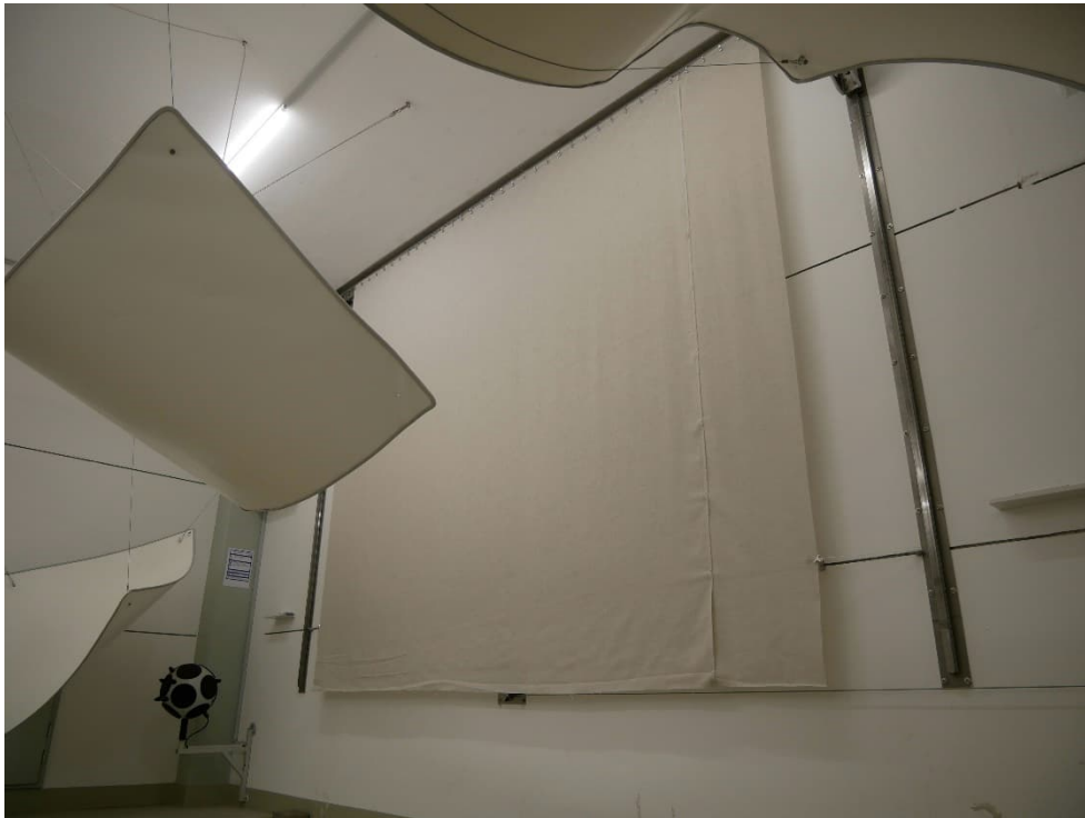
Figure B.2. Flat hanging curtain in the reverberation room: diagonal view.
