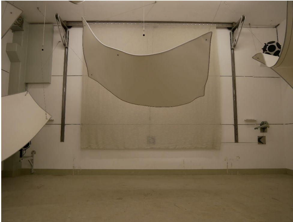
Figure B.1. Flat hanging curtain in the reverberation room: frontal view.
