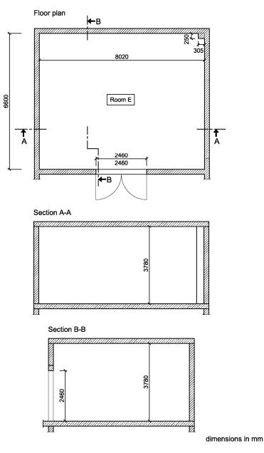
Figure C.1. Plan view and sections of the reverberation room.
