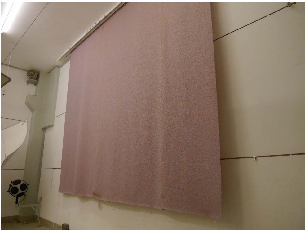
Figure B.2. Test object in the reverberation room: diagonal view.
