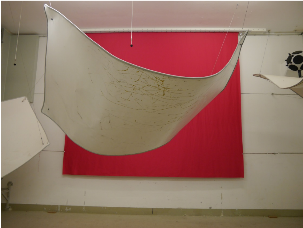
Figure B.1. Flat arrangement: test object mounted in the reverberation room, frontal view.
