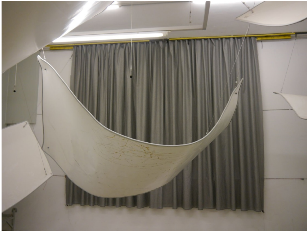
Figure B.3. Folded arrangement: test object mounted in the reverberation room, frontal view.
