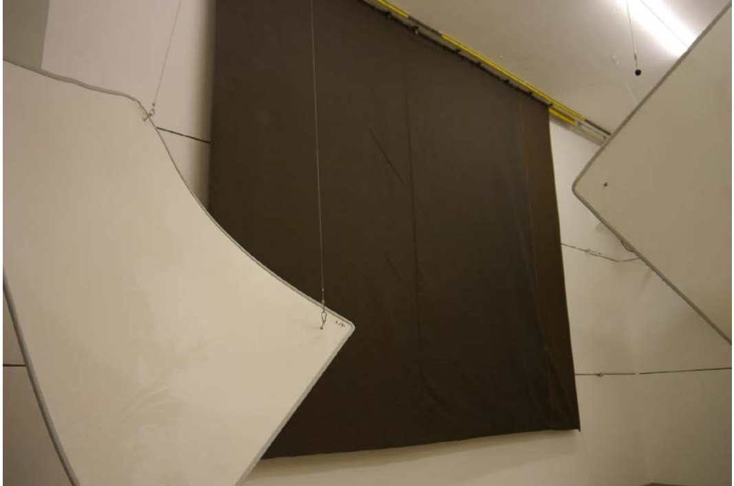
Figure B1. Flat arrangement: test object mounted in the reverberation room.
