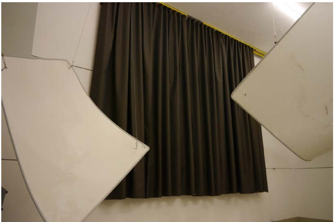
Figure B2. Folded arrangement: test object mounted in the reverberation room.
