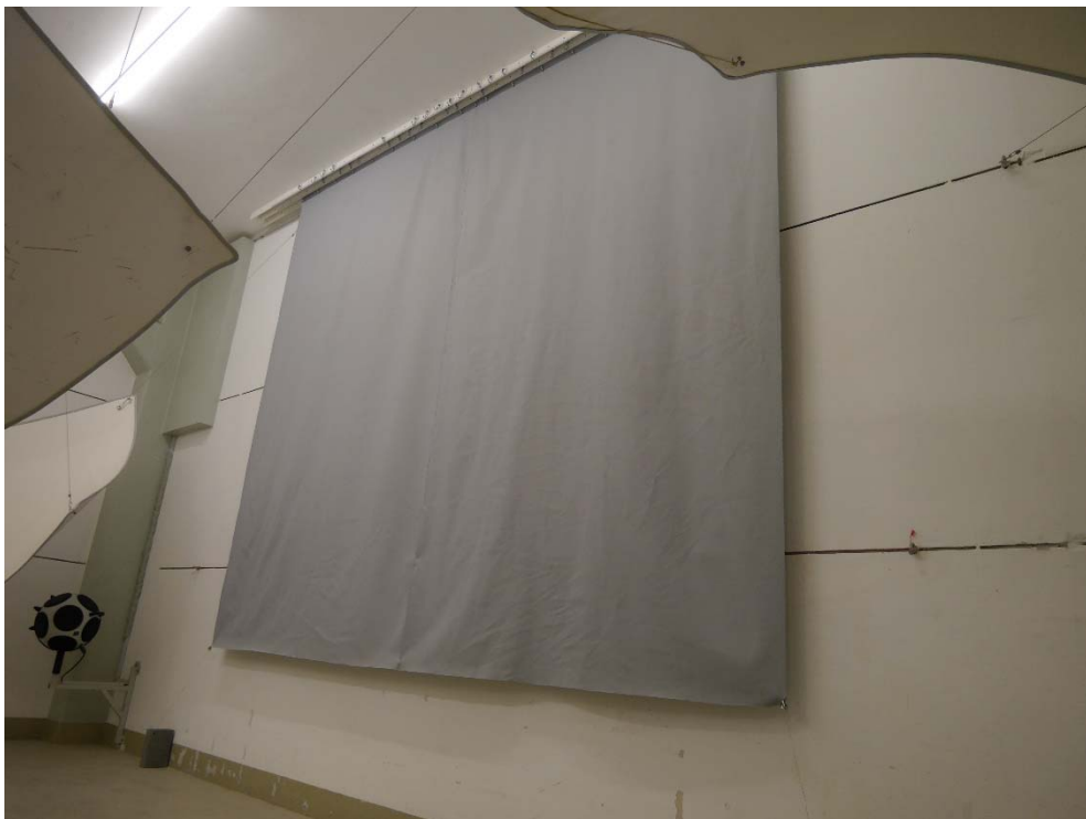
Figure B.2. Test object in the reverberation room: Flat arrangement, diagonal view.
