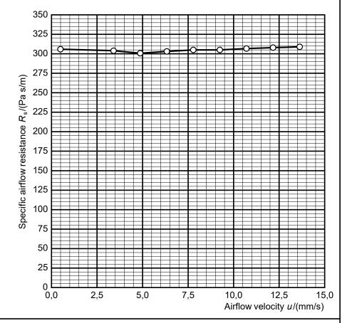
Specific airflow resistance  $R_s = 303 \text{ Pa s/m}$
