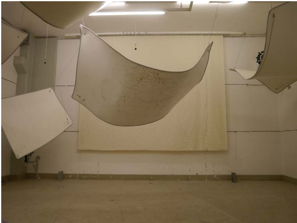
Figure B.1. Test object in the reverberation room: Flat arrangement, frontal view.
