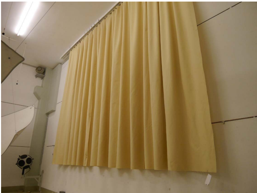
Figure B.4. Test object in the reverberation room: Folded arrangement, diagonal view.
