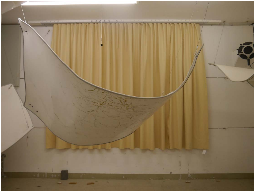
Figure B.3. Test object in the reverberation room: Folded arrangement, frontal view.
