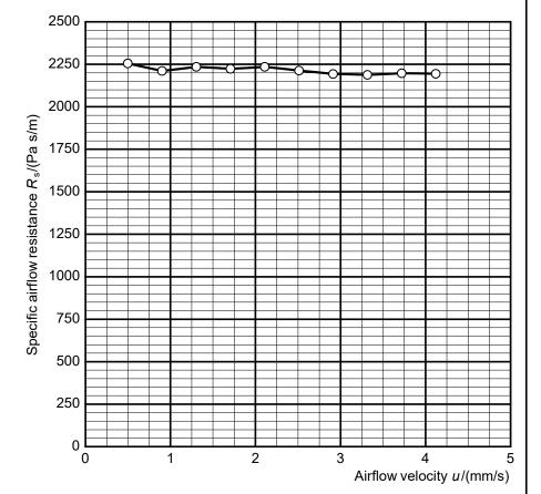
Specific airflow resistance  $R_s$  = 2241 Pa s/m
