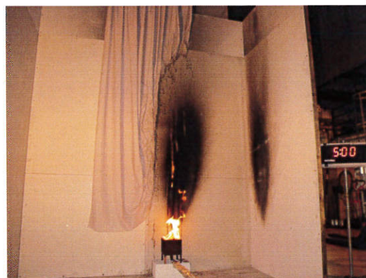
Photo 5 – Time 05:00 The burner has just been extinguished. The test is terminated.
