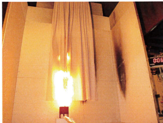
Photo 8 - Time 00:06. The burner has been ignited.
