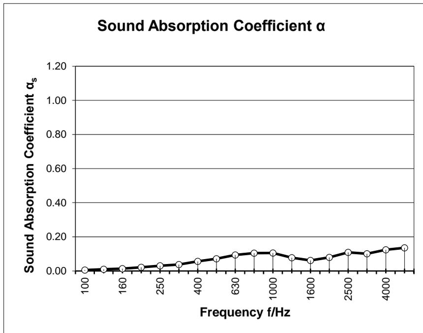
$\alpha_s$  Sound absorption coefficient to ISO 354
