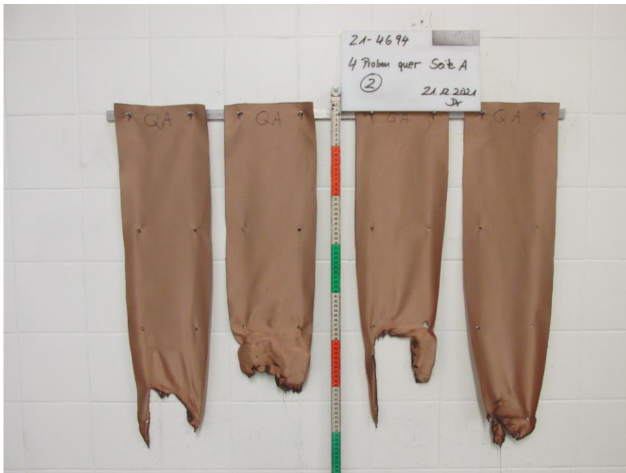
fig 2: Photo of test specimen after the test
