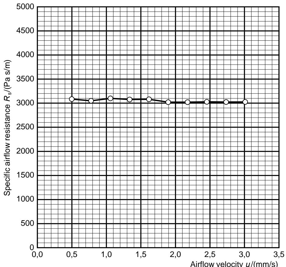
Specific airflow resistance  $R_s = 3086 \text{ Pa s/m}$
