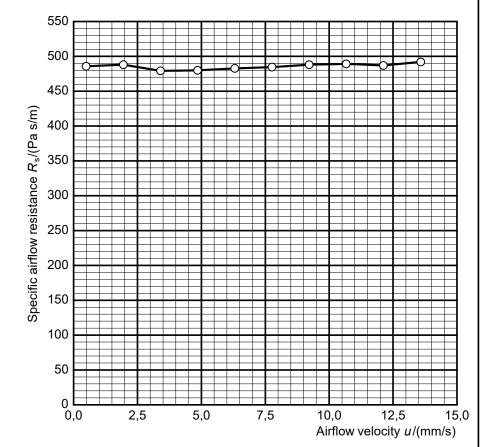
Specific airflow resistance  $R_s$  = 482 Pa s/m
